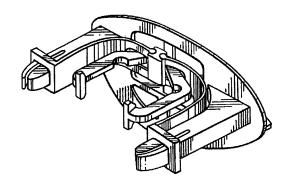
Baffle Plate, Spring and Retainer\*
