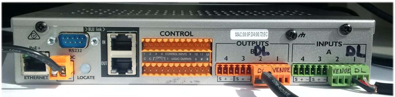
Rear View of DL-SOUNDWEB which is a pre-programmed BSS Audio BLU-50
